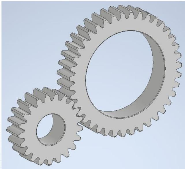
*Straight gear pair - 21x39 - transverse module 2.5mm*
