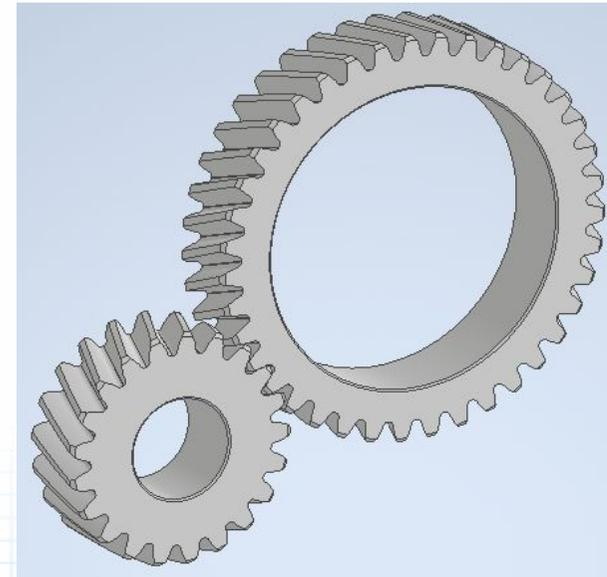
*Helical gear pair - 21x39 - transverse module 2.5 mm -
