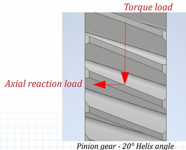
The helix angle leads to an axial reaction load. In our example, with a torque load of 800 kg, the axial reaction is 300 kg.
